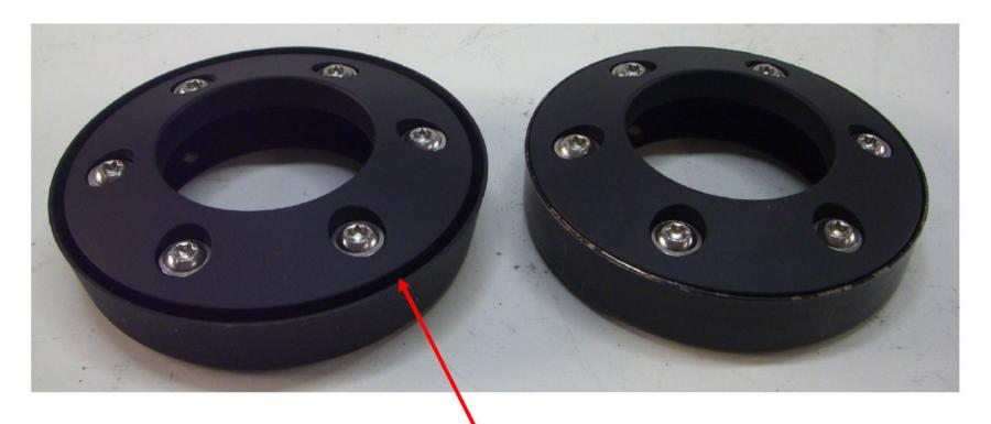
Gap of 2-3mm at models from 2003 with conical shaped end.
